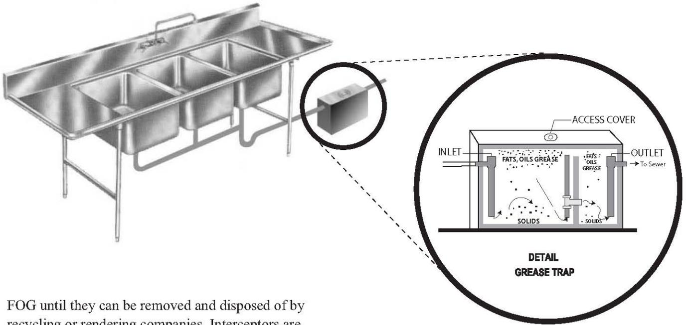
FOG until they can be removed and disposed of by recycling or rendering companies. Interceptors are more effective than grease traps and require monthly inspection and periodic cleaning.
